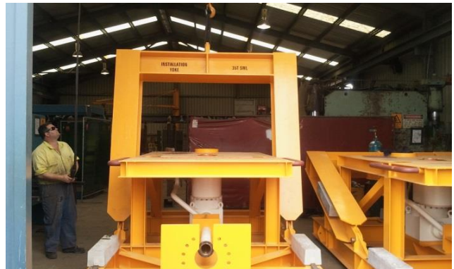
Completed PLET in Preparation for Storage
