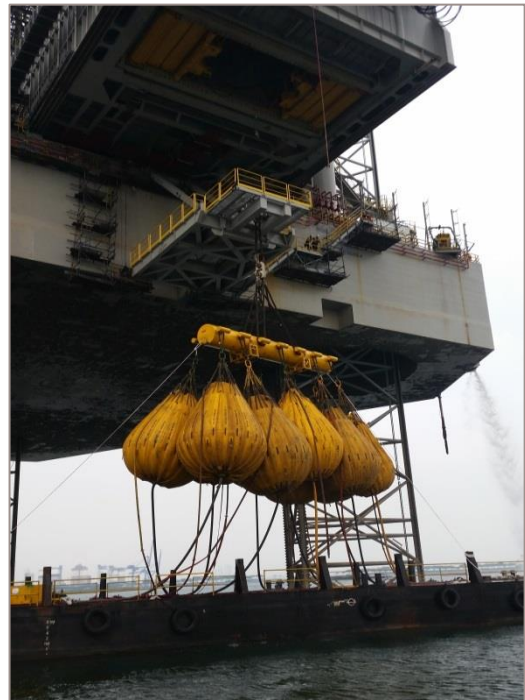
Tension Deck under 450Te load test
