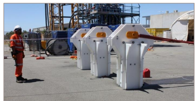
Taut wire units being tested in ICON's Henderson workshop facility
