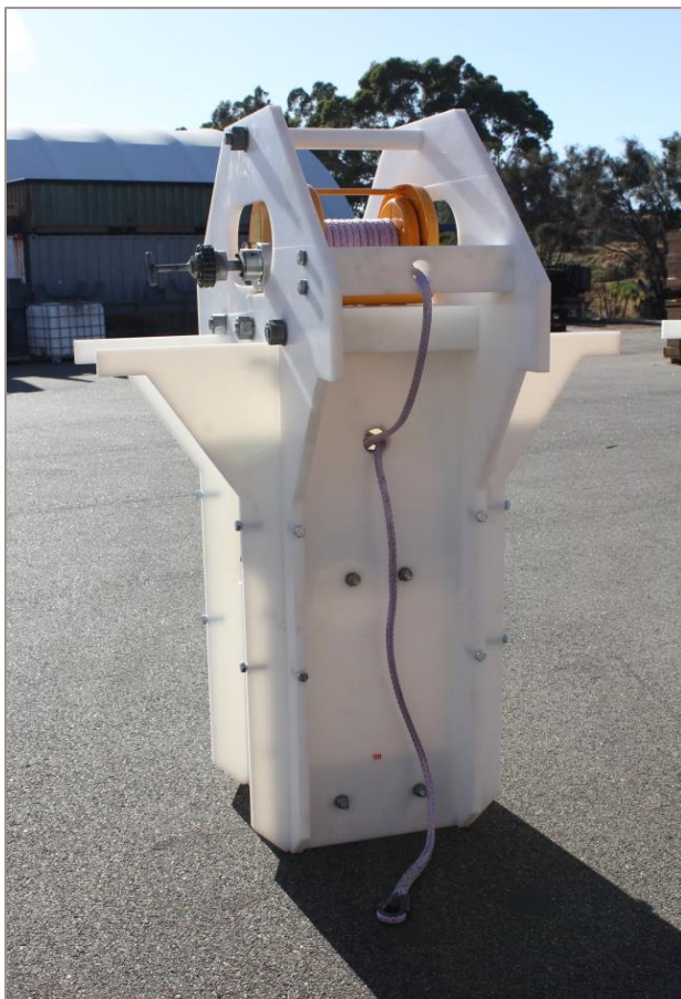
Completed taut wire unit
