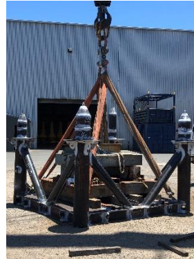
TRT Inspection and Test Stand Load Testing
