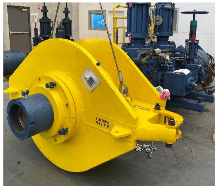
ICON Lower Spreader Beam fitted to Third Party Surface Flowhead
