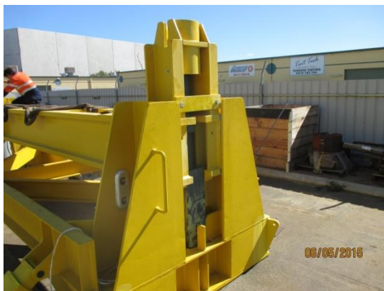
ROV Operable Jacking Screw Assembly
