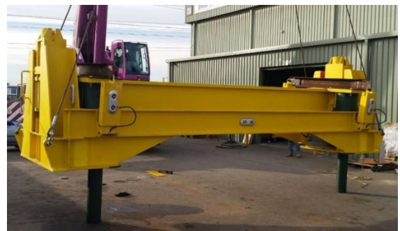
Completed PLRLS Unit: Soft Landing Cylinders Extended
