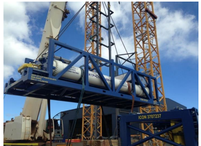
Extensive onshore testing and third party certification of the ARTP C-Series Compensated Coiled Tubing Lift Frame (CCTLF) ensured all equipment is supplied in accordance with relevant industry standards and seamlessly integrates with rig operations
