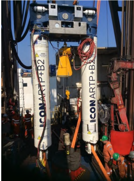
An ARTP B-Series Compensated Tension Lift Frame deployed on an Australian LNG project.
