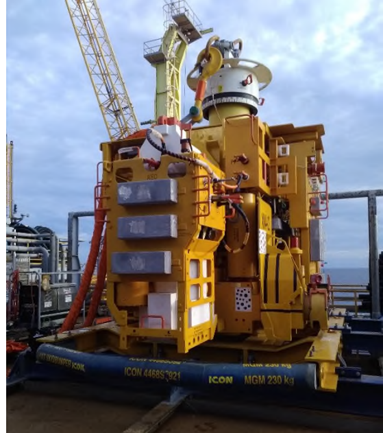
3D point cloud survey scans confirmed key clearances for the XENA 02 Xtree.
