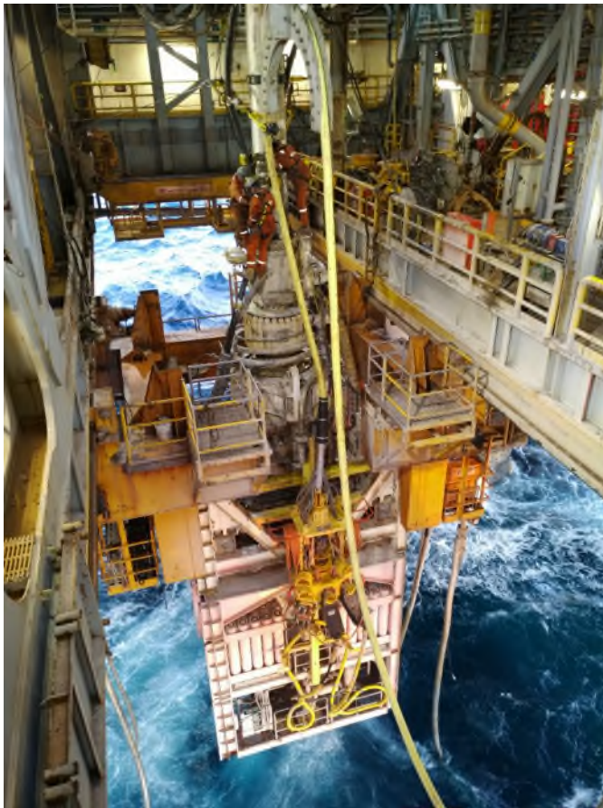
XNA-02 Tree deployed to -180m on Drill String.
