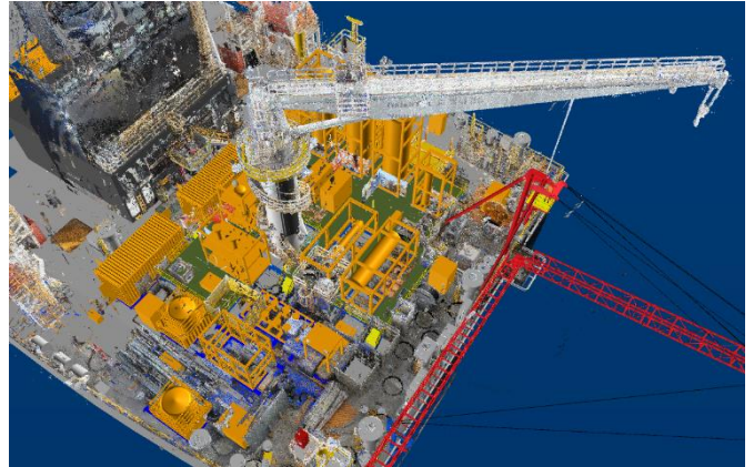
Ocean BlackRhino Well Testing Area with Burner Boom
