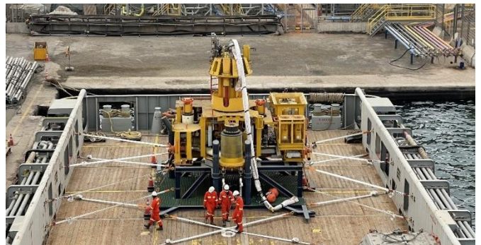
Subsea Tree installed on PSV
