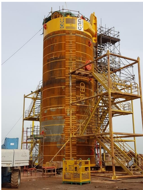
CAN positioned for low pressure well head housing integration
