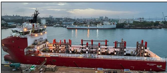
Guides Load out on Platform Supply Vessel.
