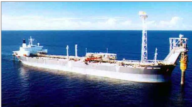
Jabiru Venture FPSO Connected to RTM
